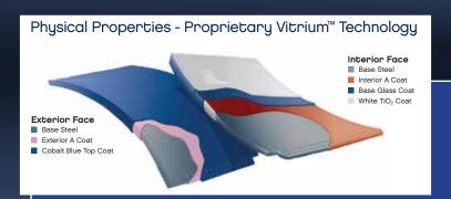
Most epoxy coatings and paint are mechanically bonded to the steel in thicknesses of 7-11 mil on the interior of the tank. The exterior thicknesses are even less, in the 6-10 mil range.
